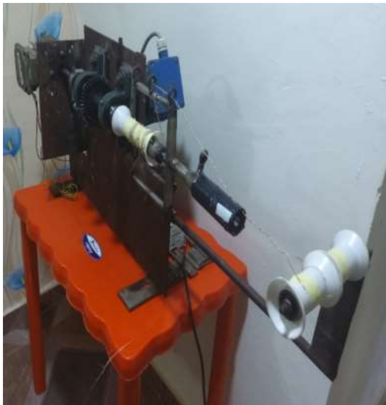
Fig. 6: Kenaf Spinning Machine (Double Ply Yarn)
